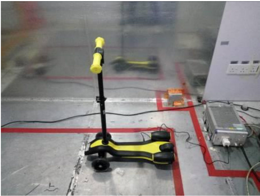
Conducted Test Setup Photograph
